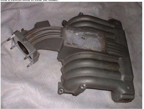
1994-95 Mustangs and 1991-93 Thunderbirds have the lowest intake profile at 9.5 inches, but to keep the intake runner length the intake is wider and contacts the master cylinder. Those intakes mount the throttle body at a 45° angle aimed towards the back of the headlight, so if the upper intake is flipped to the driver's side, the throttle body aims directly towards the brake master cylinder.
